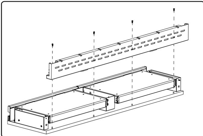
**2** Install the legs by locking into the slots provided in the side bracket.
