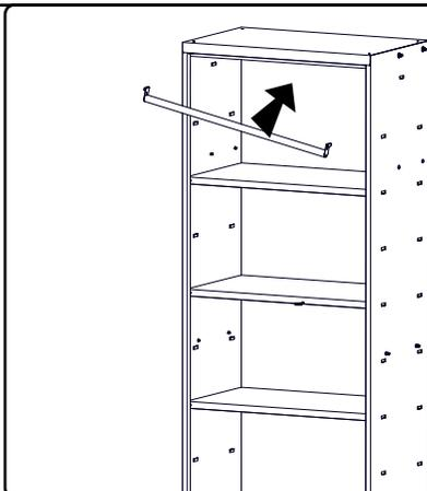
**7** Level Rod and slide down into middle slot.
