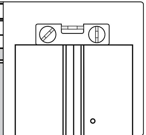
**5** Install 4 wall screws and washers through perforated holes into studs.
