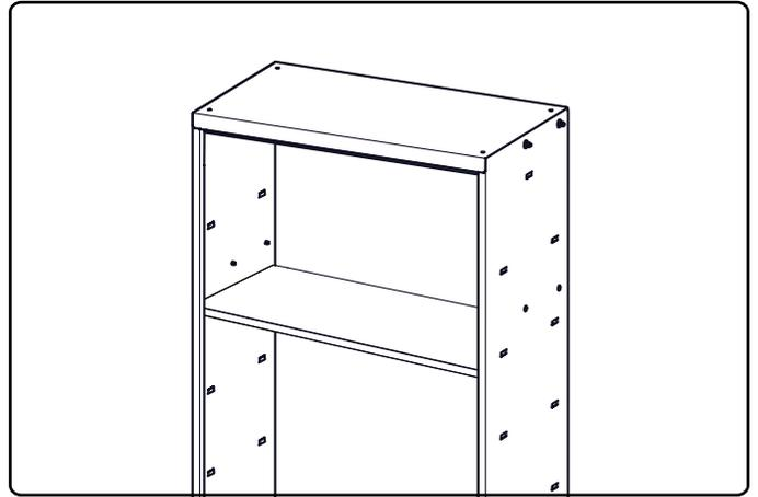
**3** Lower shelf onto brackets by sliding tabs into slots.
