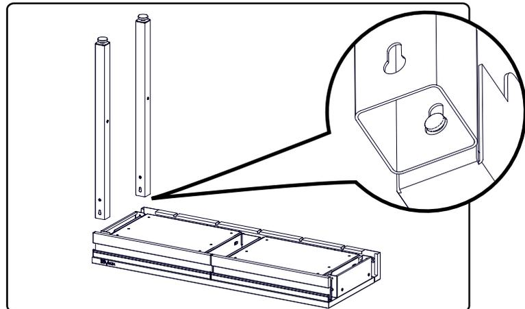
**3** Install the legs to the bracket with the screws and washers.
